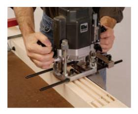
**1** Use a router and edge guide to cut the mortises in the easel legs. Then, readjust the bit depth and rout the panel grooves. Use a table saw to cut the tenons on the rails.
