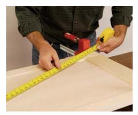
Spread glue on the frame joints and assemble the door. Apply clamps and check that diagonal measurements are equal.
