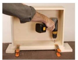
**10** Attach the bottoms with screws. Clamp each face to its drawer box and secure with screws. Then install the drawer slides.
