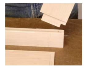
Cut the door panel from 1/2-in. plywood. Test fit the door-frame joints to make sure they're not too tight or loose.
