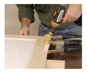
**5** Bore screwholes for attaching the trays. We used an angled block as a guide for accurate hole position and angle. Rout recesses in the trays and secure them to the frames.
