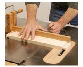
Cut the tenons with a dado blade and table saw. Use a backsaw to cut the tenon haunches (small stepped shoulders).
