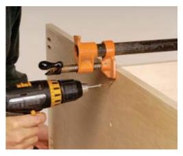
**7** Clamp sides to the bottom and drive the pocket screws. Then, lay the top upside down, position the cabinet on it and secure with screws.
