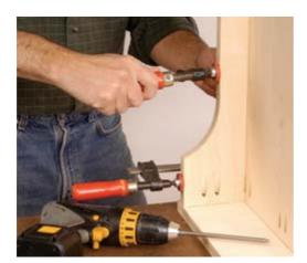
8 Use a sabre saw to shape the apron. Then, glue and screw it to the cabinet. Attach the plywood back and add the shelves.
