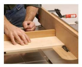
**9** Install a dado blade in your table saw and cut the rabbets in the drawer sides. Assemble the drawer boxes with nails and glue.
