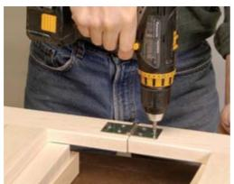
**6** Support the easel frames so they lie flat, and install the hinges at the frame tops. Then, cut the brackets to size, bore holes for the knobs and install the brackets.
