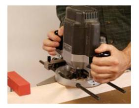
Cut maple stock for the door frame. Rout the mortises, square the rounded ends with a chisel and rout the panel grooves.
