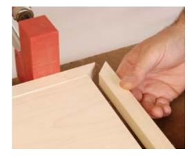
**3** Lay out the stopped rabbets in the top and side panels, and use a router to make the cuts. Square the rabbet ends with a chisel.
