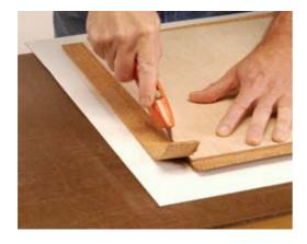
**3** Press the cork in place and trim excess with a utility knife. For the white marker board, we bought a framed board from a home center and removed the frame.
